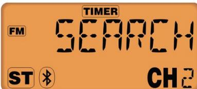
4. The unit will display a list of devices found. If more than one device is found, an arrow appears. Press **VOL+** or **VOL-** to select desired device from list.
